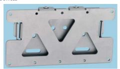
Wall mounts designed for medium sized LCD screens that have a VESA MIS-E mounting pattern of 200mm x 100mm. They can also be used to mount screens with VESA MIS-D  $100\text{mm} \times 100\text{mm}$ . Maximum weight of screen is 24kg.
