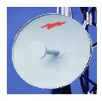
1.2 m | 4 ft Standard Parabolic Unshielded Antenna, single-polarized, unpressurized, 5.250–5.850 GHz, N Female, gray antenna, with flash, standard pack—one-piece reflector
