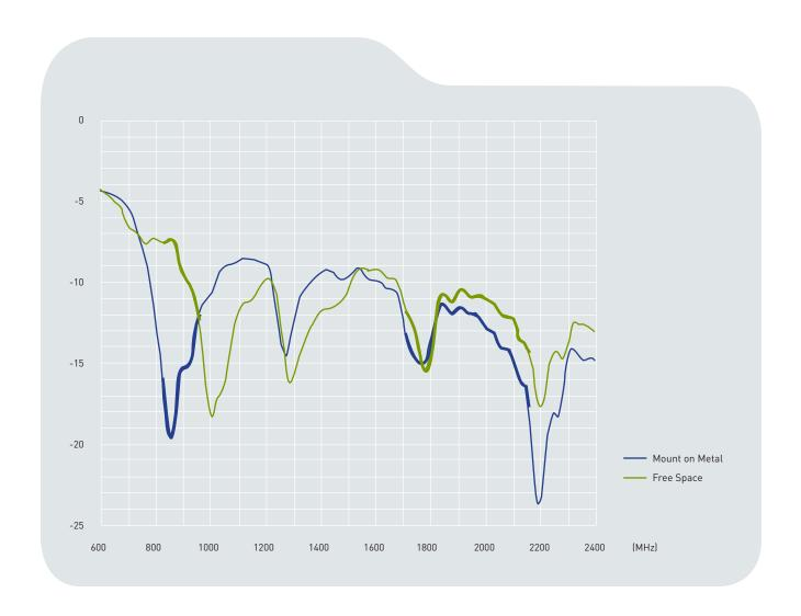
The highlighted parts are cellular operation frequency.
