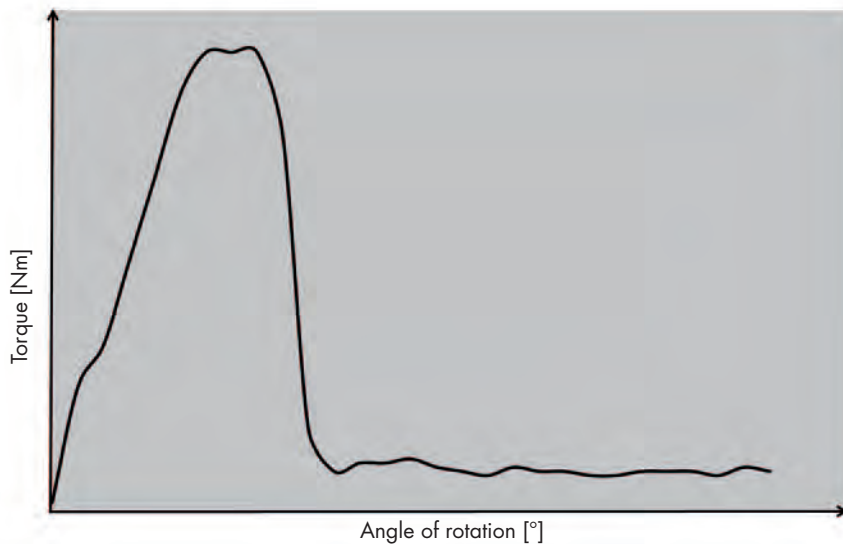
Torque-angle of rotation diagram with the stroke set correctly
