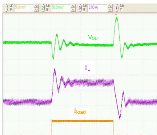
Figure 14. 500 mA to 3 A to 500 mA, 5 \mu\text{s}/\text{div} .
