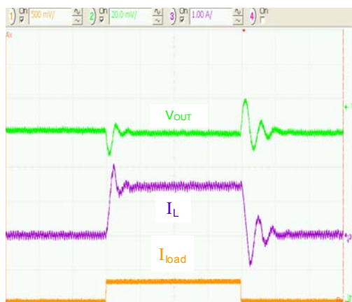
Figure 15. MODE=1, 100 mA to 1.5 A to 100 mA, 5 \mu\text{s}/\text{div} .
