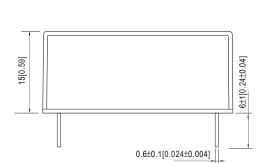
Case No.IRM02 Unit:mm[inch] Tolerance:±0.5[±0.02] unless otherwise specified
