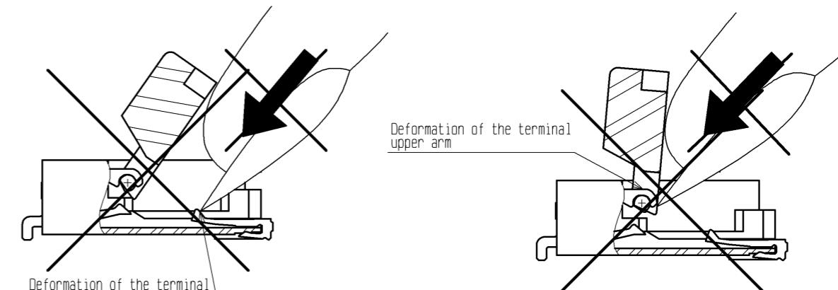
2. The actuator rotates around the rotational axis as shown below.
