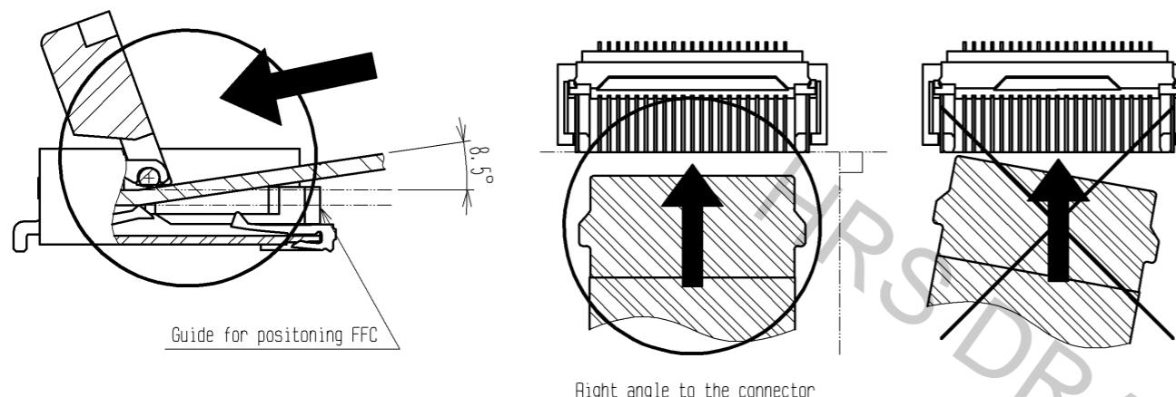
2. Do not insert the FFC diagonally from above.
