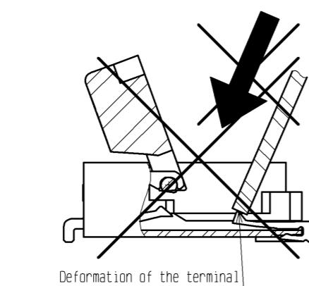
3. Do not rotate the actuator when FFC TAB is on right and left guides for positioning FFC. Make sure the position of FFC TAB and guides before rotate the actuator.
