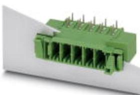
Feed-through header, nominal current: 41 A, rated voltage (III/2): 630 V, nominal cross section: 6 mm<sup>2</sup>, number of positions: 4, pitch: 7.62 mm, color: green, contact surface: Tin, mounting: Wave soldering, pin layout: Linear pinning, solder pin [P]: 4.26 mm
