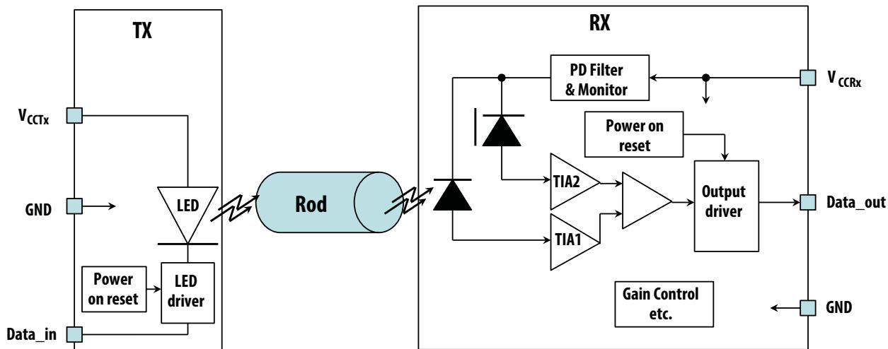
A low Input signal at Data\_in results in a low output signal at Data\_out (non-inverted Tx to non-inverted Rx).
