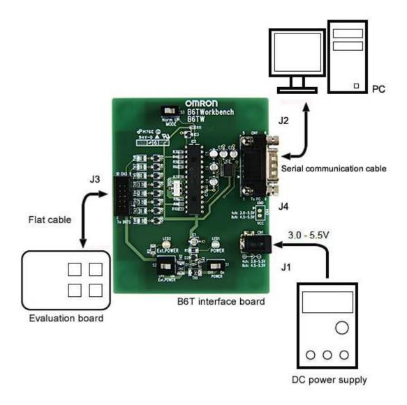
Evaluation board for eight channels (supplied with B6TW-S08NF)
