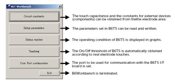
The first screen (below), circuit constraints, lets the user determine the physical constants, of the appliance control design. By entering the pad size, line length, thickness of the panel, and permittivity (material) of the panel, the two fixed capacitors ( $C_r$  and  $C_c$ ) can be established. In addition, the fixed resistance,  $R_c$  is calculated.
