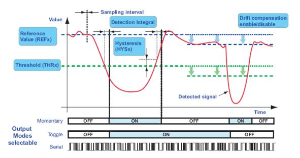
The graph below is what can actually be seen in the development program using the Status Monitor, as shown in the first Workbench menu selection. The Status Monitor allows for the user to see how the touch sensors are performing, in real time. Thus, when developing a control for an appliance, such a refrigerator, the actual switch sensing can be observed in real-time. Also, several prototypes can be used, in order to test user variations.
