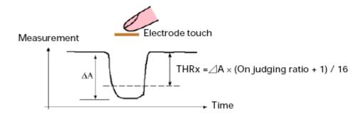
The below is a more detailed description of parameters, in a graphical setting. The red solid line is a representation of what is happening to the capacitance. The **Reference value** (REFx) is the top dotted blue line, and the **Threshold level** (THRx) is the green dotted line. The detection integral can be relayed to the delay time, of response. The sampling integral is typically in the hundreds of kHz.
