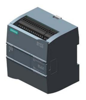
SIMATIC S7-1200, CPU 1211C, COMPACT CPU, DC/DC/RELAY, ONBOARD I/O: 6 DI 24V DC; 4 DO RELAY 2A; 2 AI 0 - 10V DC, POWER SUPPLY: AC 20.4 - 28.8 V DC, PROGRAM/DATA MEMORY: 30 KB
