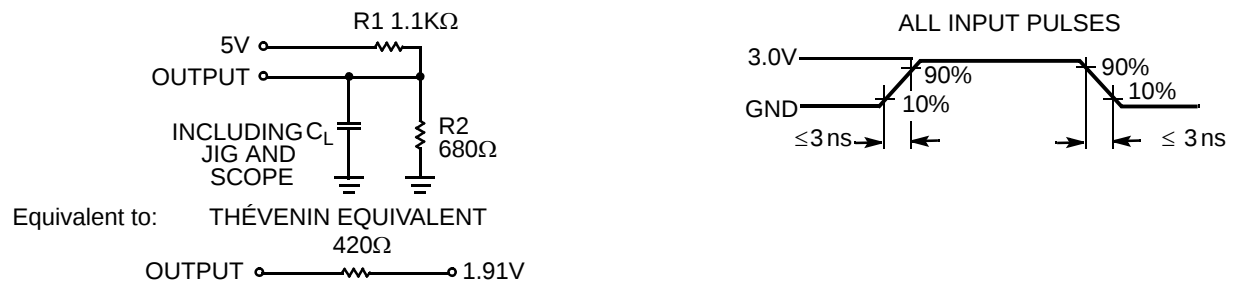
Figure 5. AC Test Loads and Waveforms [10, 11]
