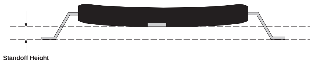
Figure 7-1. Standoff Height Measurement on 144-Pin RFP Package
