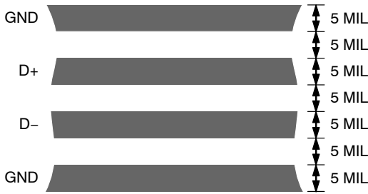
Figure 21. Typical Arrangement of Signal Tracks
