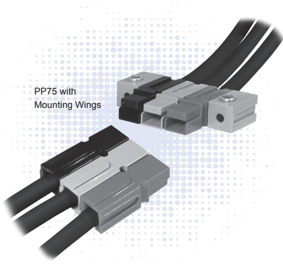
PP75 series Powerpole® housings can be used for wire-to-wire, wire-to-board, and wire-to-busbar applications. Wire sizes from #16 AWG (1.3 mm<sup>2</sup>) to #6 (13.3 mm<sup>2</sup>) offer power capabilities up to 120 amps per pole. Locking housings offer the capability to secure Powerpole® housings to each other and to mounting pads. Housings made from chemical resistant (CR) resin withstand industrial solvents better than standard housings.
