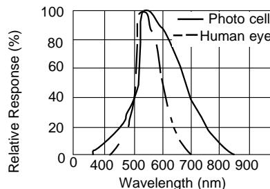
The spectral response characteristics of a cell indicates the ratio between the cells sensitivity to a light source of specific wavelength and the cells maximum sensitivity. Also color temperature error is given in the equation.
