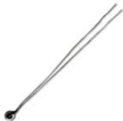
192 Series, Uni-Curve with bare leads and epoxy, 1,000 Ohm resistance,  $\pm 1,0$  °C [1.8 °F] tolerance, 25/85 BETA = 3348
