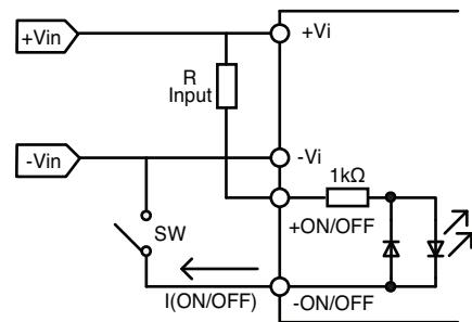
(B) Turning output ON and OFF from the output side, recommended R value is 5.1k (0.1W).
