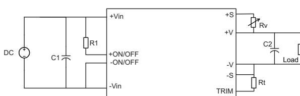
The Trim pin should be left open if trimming is not being used. The output voltage can be determined by the following equations:
