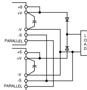
**(d) N+1 redundant connection adjustable output voltage**
