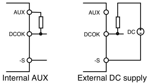
This signal is LOW when the converter is operating normally and HIGH when the converter is disabled or when the converter is operating abnormally.
