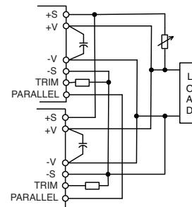
**(c) N+1 redundant connection**
