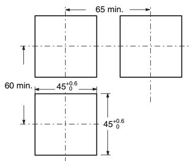
**Note:** 1. Recommended panel thickness is 1 to 5 mm.
