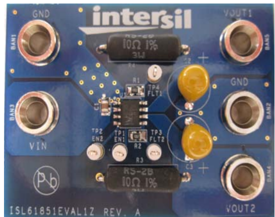
FIGURE 32B. ISL61851EVAL1Z BOARD PHOTO
