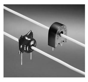
Designed for use at 20 kHz to 50 kHz and higher, these sensors function as the secondaries of a current transformer. The conductor carrying the current to be measured is the "one turn primary." Sensitivity can be set at 1 Volt per Ampere or at other desired values. It can also be doubled by looping the conductor through the hole twice. Applications include sensing branch circuit overload, switcher feedback, and detecting load drop or shutdown.
