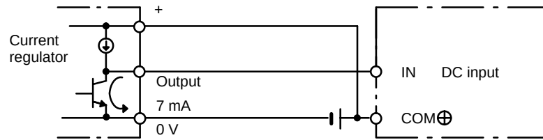
NPN open-collector output
