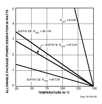
$$P_D = (V_{OUT1} \times I_{OUT1} \times dc) + ... + (V_{OUTn} \times I_{OUTn} \times dc) + (V_{CC} \times I_{CC}) = (T_J - T_A)/R_{\theta JA}$$
