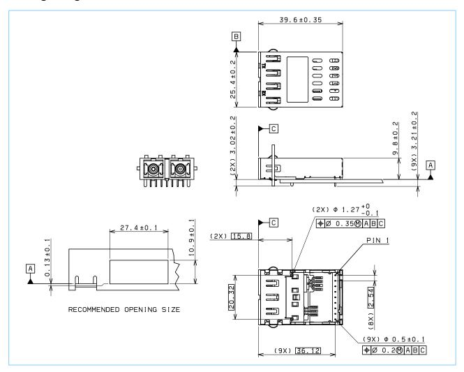
The 1X9-1063/1250-SW is intended to be used on a host card having a thickness of 0.062" to 0.100".
