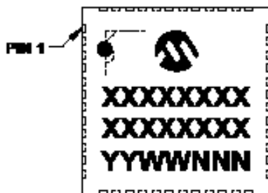
48-Lead UQFN (6x6x0.5 mm)
