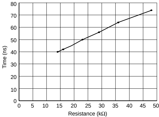
Figure 6. GATE Non-Overlap Time vs. DLYSET Resistance
