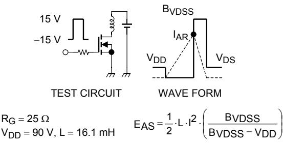
$$R_G = 25 \Omega \quad V_{DD} = 90 \text{ V}, L = 16.1 \text{ mH} \quad E_{AS} = \frac{1}{2} \cdot L \cdot I^2 \cdot \left( \frac{B_{VDSS}}{B_{VDSS} - V_{DD}} \right)$$
