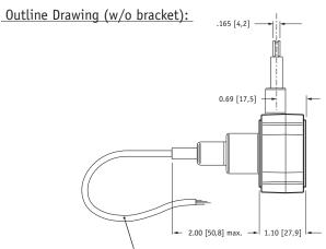
Electrical Cable, 24 GA, 3 conductor, shielded 40 in. [1 meter] long
