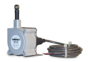
The SP3 from Celesco is a compact, economical stringpot that provides a user selectable 4-20 mA or 0-10 Vdc output signal. Simply install this sensor using the handy mounting bracket and connect the appropriate wires for the desired ouput.
