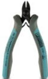
ESD electronic diagonal cutter, round head, without chamfer, with opening spring, non-reflective coating and phosphate-treated, 2-component handle, cutting capacity diameter: soft 0.2 ... 2.0 mm; medium hard 1 mm, type of packaging: with holder for sales display (backcard)
