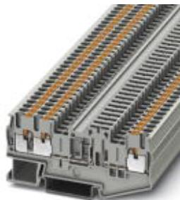
Disconnect terminal block, Connection type: Push-in connection, Cross section: 0.14 mm<sup>2</sup> - 4 mm<sup>2</sup>, AWG: 26 - 12, Nominal current: 16 A, Nominal voltage: 400 V, Length: 81.9 mm, Width: 5.2 mm, Color: gray, Assembly: NS 35/7,5, NS 35/15
