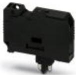
Fuse plug, Connection method: Plug connection, Nominal current: 10 A, Nominal voltage: 630 V, Width: 8.2 mm, Fuse type: G / 6,3 x 32, Fuse type: Glass / ceramics / ..., Mounting type: Plug-in mounting, Color: black
