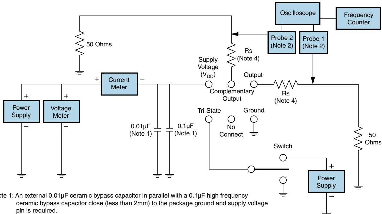
Note 1: An external 0.01μF ceramic bypass capacitor in parallel with a 0.1μF high frequency ceramic bypass capacitor close (less than 2mm) to the package ground and supply voltage pin is required.
