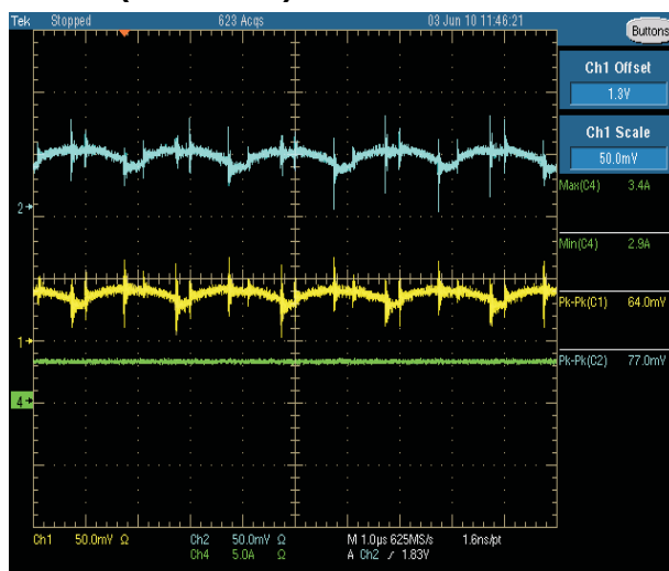
Figure 10. Ripple for Buck 1 (Yellow Trace) 1.2 V, 3 A and Buck 2 (Blue Trace) 1.8 V, 2 A, 50 mV per Division V_{IN} = 12 V, f_{SW} = 500 kHz, L_O = 4.7 \mu H, DCR = 10 m \Omega , C_O = 22 \mu F
