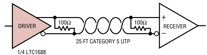
Figure 12. 100Mbps Differential Data Connection
