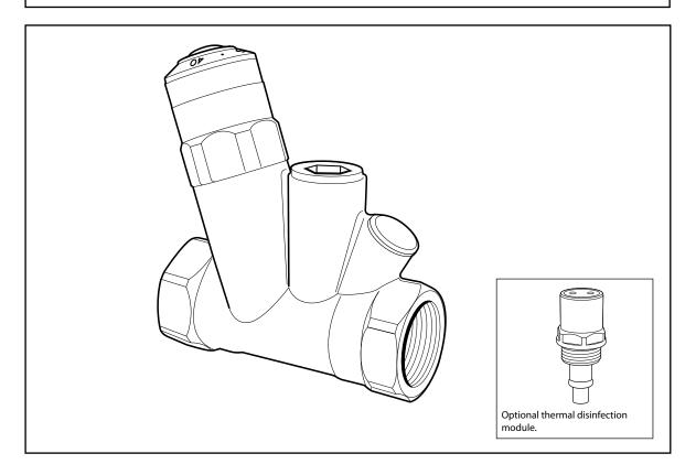
Valve for thermostatic regulation within a hot water circulation system.
