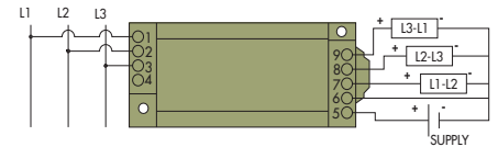
CR4860 3 Element, 3 Wire - 4-20 mA DC Output
