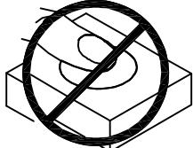
3. Do not stack together assembled PCBs containing exposed LEDs. Impact may scratch the silicone lens or damage the internal circuitry.
