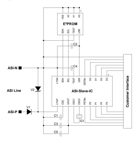
C1 = 22...470 nF / max. AS-Interface BUS DC voltage
