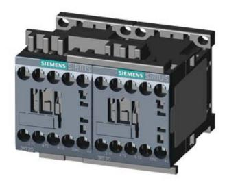
REV. COMB., AC3, 7.5KW/ 400V AC110V 50HZ/120V 60HZ 3-POLE, SZ S00 SCREW TERMINAL ELECTR. AND MECH. INTERLOCK
