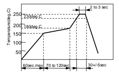
IR REFLOW SOLDERING
