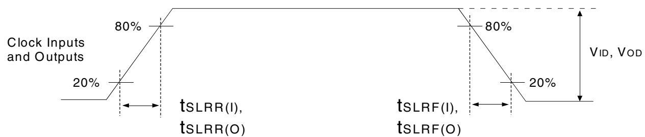
Figure 8. Input and Output Slew Rates
