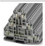
Multi-level terminal block, Cross section: 0.2 mm² - 10 mm², AWG: 24 - 8, Connection type: Screw connection, Width: 8.2 mm, Color: gray, Mounting type: NS 35/7,5, NS 35/15
