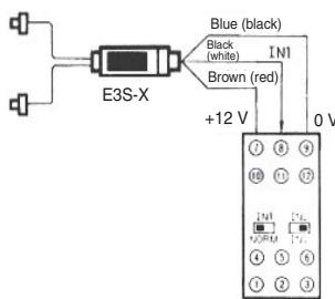
Note: A maximum of two S3D2 Sensors can be connected.
