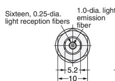
Note: The fiber for the emitter is identified by a white line.
