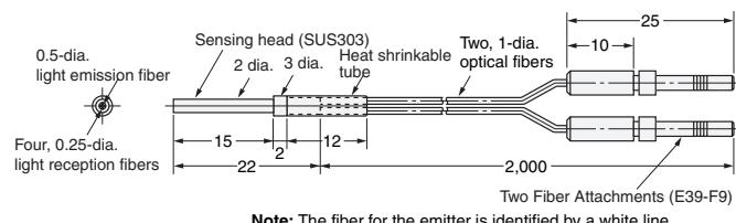
Note: The fiber for the emitter is identified by a white line.
