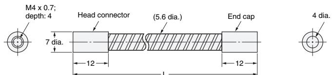
**Note:** The length L is 1,000 for the E39-F32C and 500 for the E39-F32C5.
