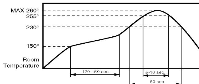
**WAVE SOLDERING:** 260°C maximum solder temperature for 5 seconds max.
