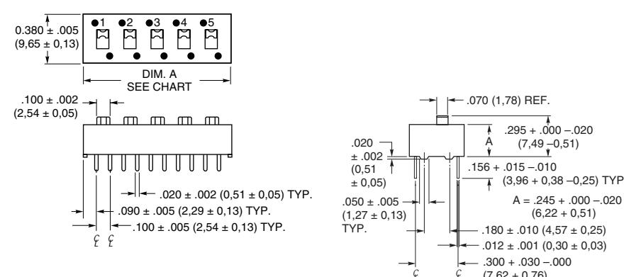
**CIRCUITRY: Series 78****SPDT, 2 Circuits (No Commons)**
