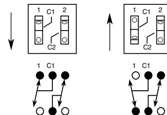
**DIMENSIONS: Series 78** In inches (and millimeters)**Series 78 Slide**
