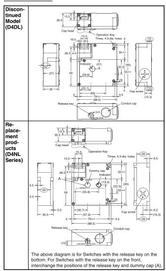
Differences: The depth of the M4 mounting screw holes is 29 mm for the D4NL, as opposed to 10 mm for the D4DL. Therefore, when replacing the D4DL with the D4NL, use M4 screws that are 19 mm longer than the ones used before.
