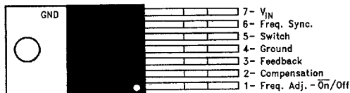
Bent, Staggered Leads 7-Lead TO-220 (T) Top View
