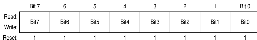
Figure 14-8. TIM Counter Modulo Low Register (TMODL)
