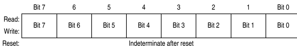
Figure 14-13. TIM Channel Register Low (TCHxL)
