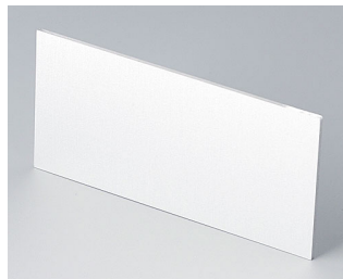
B6132111 Front panel Aluminum matt anodized 3.60"x1.71"x0.06"
