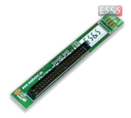
Adapter to connect SlimLine CD / DVD drives to classical IDE44 / PATA / P-ATA controllers.
