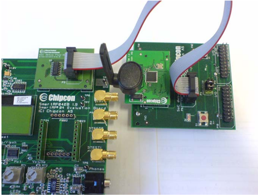
Figure 9: SmartRF04EB to program SOC_BB
