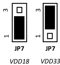
Figure 3-2. VDDIO Select (JP7) Jumper Settings
